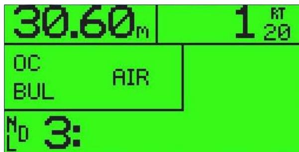
Figure 21: Main Screen in Dive Mode Open Circuit - Mix: Air No Deco Time 3 minutes
