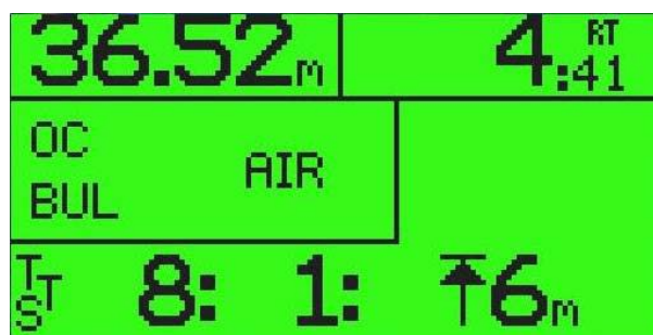
Figure 23: Main Screen in Dive Mode Open Circuit – Mix: Air Deco Stop at 6 meters for 1 minutes Time To Surface 8 minutes
