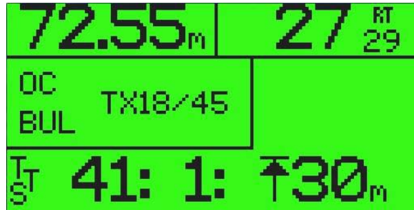
Figure 26: Main Screen in Dive Mode Open Circuit – Mix: Trimix 18/45 Deco Stop at 30 meters for 1 minute Time to Surface 415 minutes
