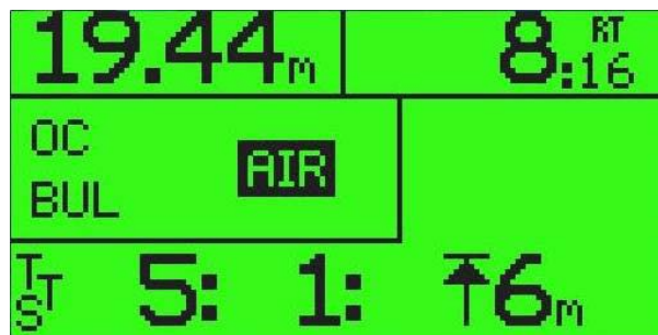
Figure 24: Main Screen in Dive Mode Open Circuit – Mix: Air Deco Stop at 6 meters for 1 minute Time to Surface 5 minutes Mix Change Warning
