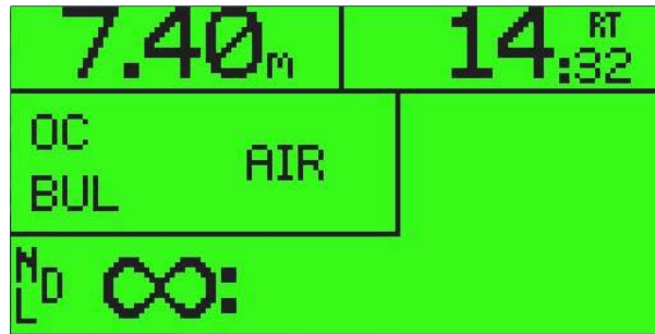
Figure 22: Main Screen in Dive Mode Open Circuit – Mix: Air No Deco Time more than 99 minutes
